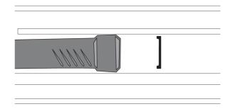
Place a small block of 2X4 wood in Jamb channel. Butt against the male tab which has been pushed through and hammer.
