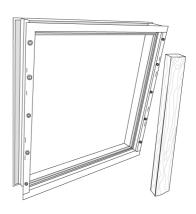
Nail through center of head into wood brace on both the top and bottom of buck for delivery to job site.
