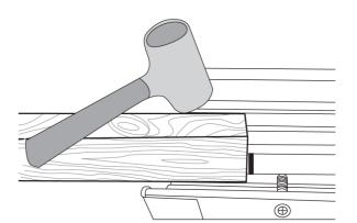
Be sure to look for the tooth on the male tab, which will kick out and lock in place leaving tab vertical.
