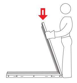
Before installing remaining Jamb, make sure that corners of the Jamb are tucked slightly to allow for overlap from Sill.
