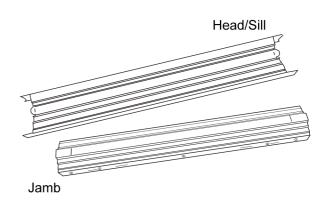
Tilt Sill at a 45 degree angle and insert end tab into Jamb slot using downward pressure.
