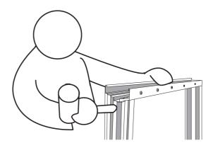
Be sure that you have proper overlap and alignment of Sill and Jamb.
