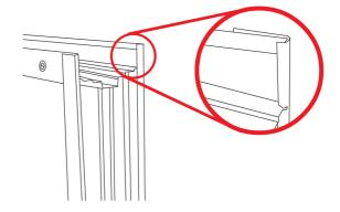
Repeat the previous steps on the opposite end of Sill. Lift and rotate entire frame and repeat these steps again making sure all four corners are properly seated.
