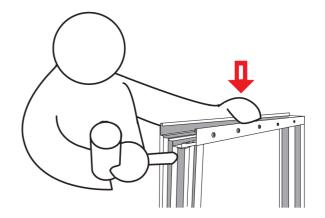
Use end of a mallet to straighten tab back to a vertical alignment of 90 degrees.
